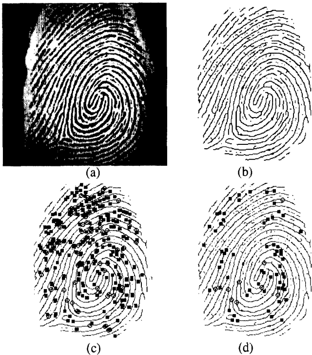
Figure 5. Example of minutiae validation when the image is segmented using a local threshold: the original image (a), the thinned ridge map image (b), the candidate minutiae over the thinned ridge map image (c), and the valid minutiae over the thinned ridge map image. The ridge endings and ridge bifurcations are marked with squares and circles respectively.
