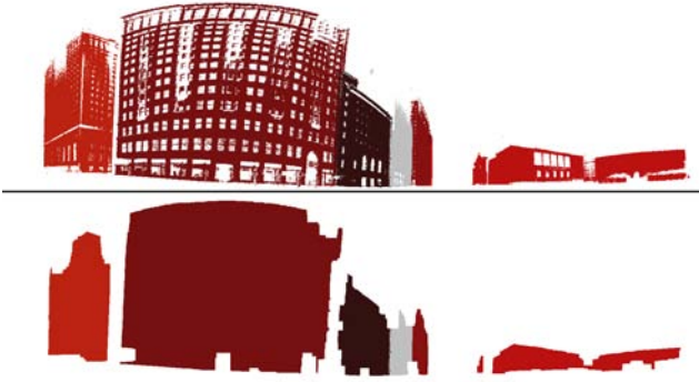
Figure 3. Point cloud is first projected to the image, holes are filled and finally the result is eroded slightly to avoid false labeling background as buildings. Top half shows the original projection, and lower half the final result.
